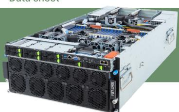
HPC/Al Server - 4th/5th Gen Intel® Xeon® Scalable - 5U DP HGX™ H100 8-GPU | Application: Al , Al Training , Al Inference , Visual Computing & HPC
